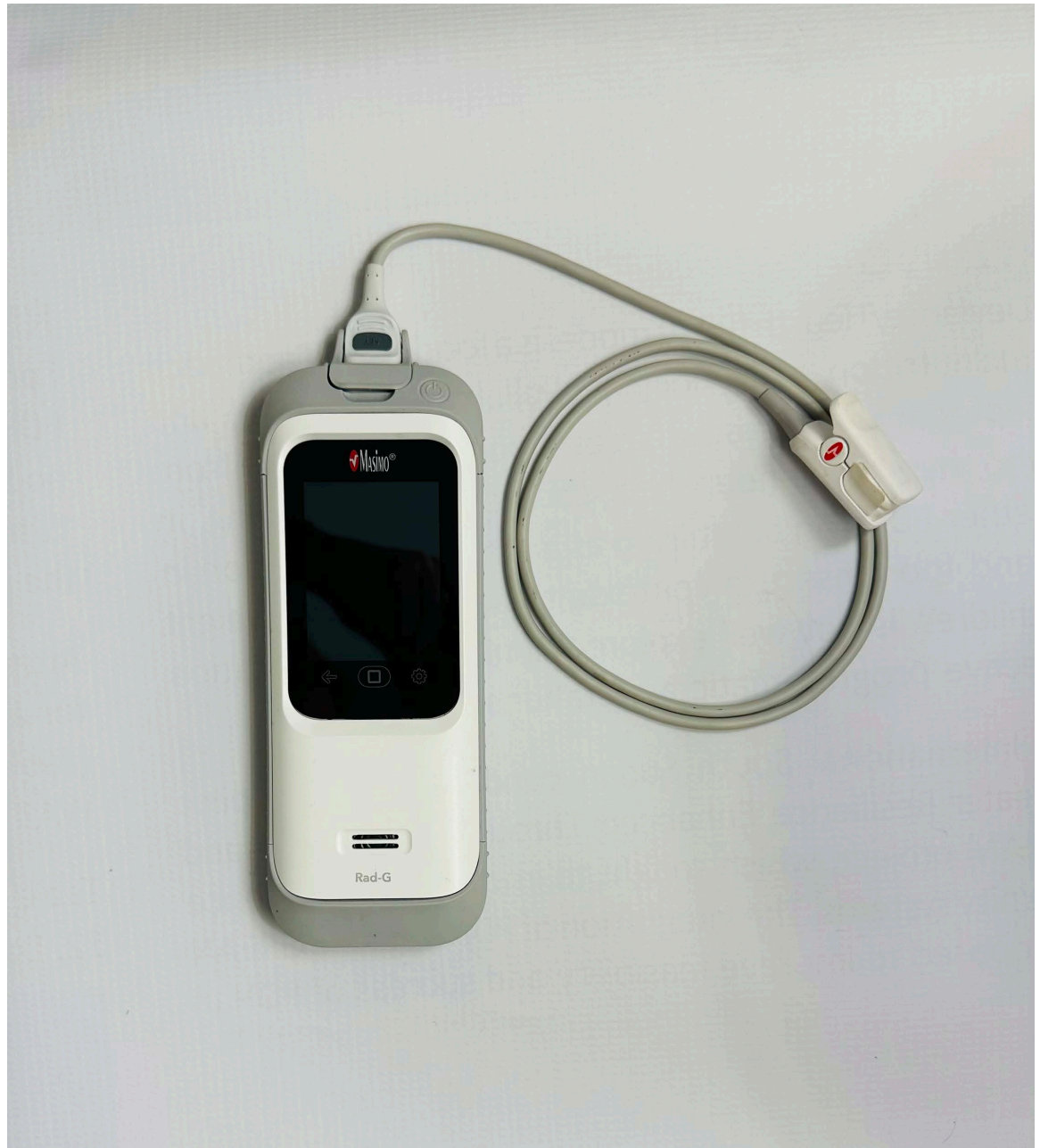
Fig 1. Masimo's Rad-G pulse oximeter and reusable clip probe (sensor) used by CHWs during their iCCM consultations.
